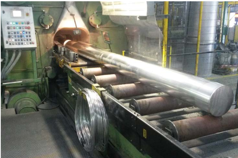
5500-T Indirect extrusion press
