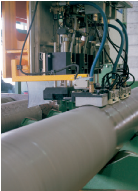
Automatic ultrasonic control system for the entire length of the billet according to class "A" of SAE AMS-STD-2154 regulation
