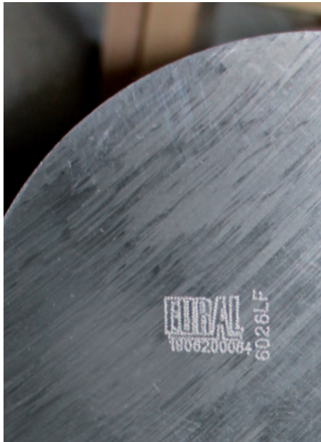
Imprint of Eural logo, alloy code and batch number on all extruded bars
