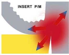
The inserts commonly called N and designed specifically for machining aluminium have a rake angle that does not allow an appropriate and sufficient distribution of heat during turning. Therefore, chip breaking is compromised, forming long and curled chips.
