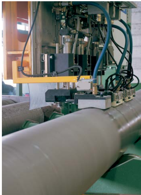
Automatic ultrasonic control system for the entire length of the billet according to class "A" of SAE AMS-STD-2154 regulation
