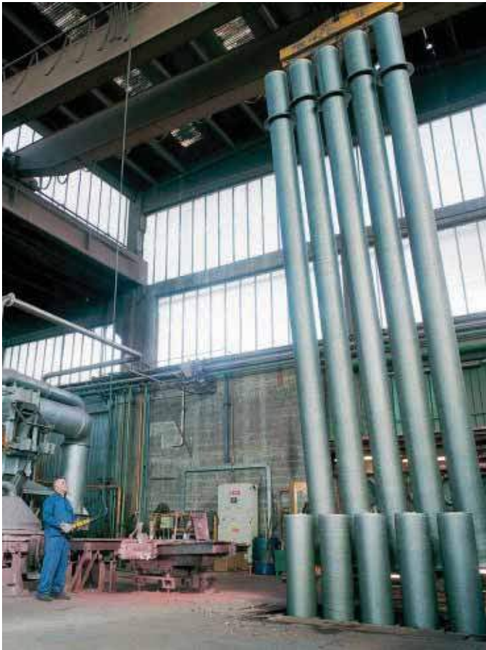
Billets extraction in foundry
