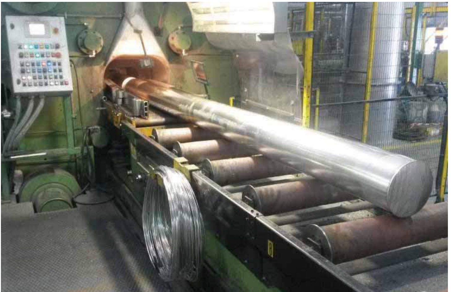
5500-T Indirect extrusion press
