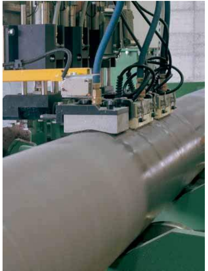
Automatic ultrasonic control system for the entire length of the billet according to class "A" of SAE AMS-STD-2154 regulation
