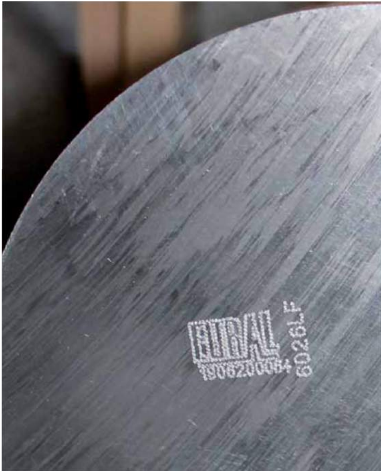
Imprint of Eural logo, alloy code and batch number on all extruded bars
